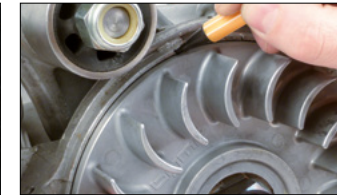
Turn the flywheel clockwise until it rests against the piston stop and then mark it on the maghousing
