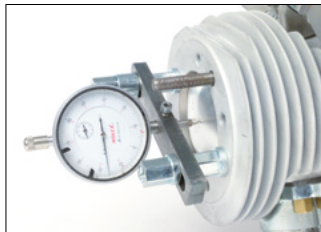
Dial gauge fitted with our bracket and cylinder nuts used as packers
