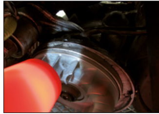
Now you can fire the engine up and strobe the ignition timing settings. Hold the strobe gun to your TDC marking and have a look at the flywheel timing marks to see your actual ignition timing. If you are happy with the setting, you can start to wire the electrical system.
