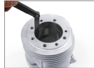
Use the feeler gauge to measure the ring gap
