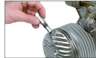
Fitting the piston stop instead of spark plug
