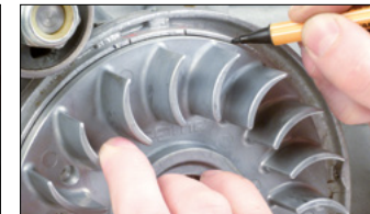
Turn the flywheel anti clockwise until it rests against the piston stop and then mark it on the maghousing
