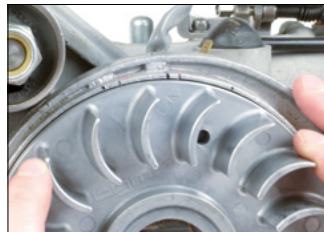
Once you found the TDC using the dial gauge you can mark this opposite to the arrow on the flywheel
