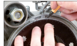
Use a soft ruler or a timing degree disc to find the middle between the two positions. This is your Top Dead Centre (TDC).
